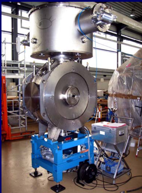
9.6 T superbend designed and produced in the Budker INP for BESSY-II (2004)
